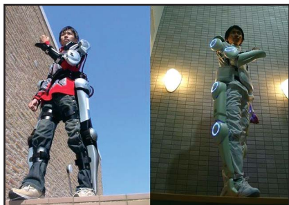
The HAL exoskeleton power assist system, worn by Prof. Sankai. Photo courtesy of Cyberdyne, Inc.
